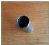
It's 50mm long and it has an exact diameter of 18.95mm.
